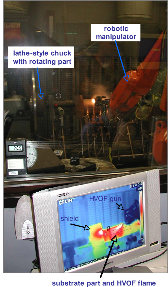
Fig. 1. Thermal image of component during spraying as seen from HVOF operator's control room.
